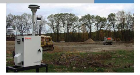
The Thermo Scientific Partisol 2000-D Dichotomous Air Sampler is a single-event particulate matter (PM) sampler that holds two filters for the simultaneous collection of the fine and coarse particles contained in PM-10.
